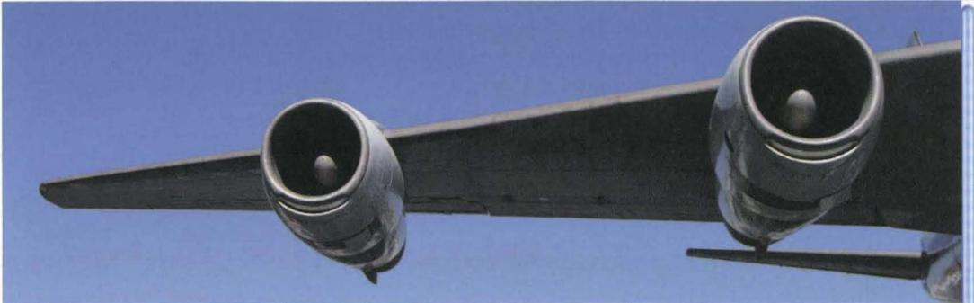
**Aluminium** is widely used, often in alloy forms. An example is duralumin, an alloy used in aircraft manufacturing, which also contains **copper** (4.4%) and **magnesium** (1.5%). Aluminium can also be alloyed with **titanium** to produce very strong, lightweight metals.
