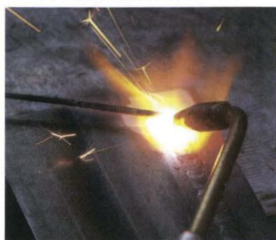
Gas welding using oxyacetylene
