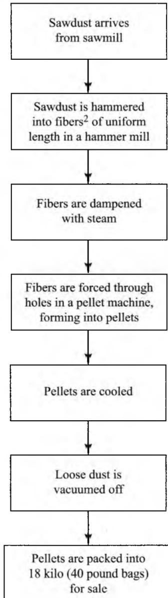
Wood pellets manufactured by this process are suitable for use in both pellet stoves and pellet furnaces.
